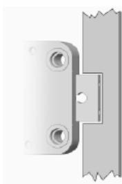
In the LOCKED position, there should be approximately 1 mm clearance between the lock bolt and the cavity in the blocking bar of the boltwork. The lock bolt must move freely into the cavity.
