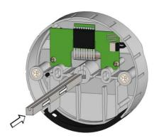
Fix the screws (M4) and the rotating backplate, positioning the latter on the side marked "UP". Fix the bushings to the keypad housing using the supplied screws.
