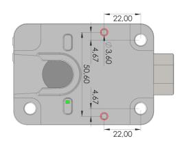
Fix the relocker plate with M4 self tapping flat head screws. Length must be 6mm + plate thickness.
