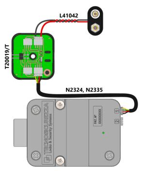
Different and customized items not provided by Tecnosicurezza, may also work provided they supply the voltage to the cables black and yellow of connector 1.
