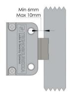
In depending of the motor lock type, the distance between the lock and the locking edge must be between a minimum of 6 mm and a maximum of 10 mm.
