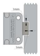
In the locked position, there should be approximately 1 mm clearance between the lock bolt and the cavity in the blocking bar of the boltwork. The bolt must be able to move freely without applying any force on it.
