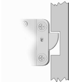
In the LOCKED position the distance between the MiniRotobolt bolt and the MiniRotobolt part that is moving the lock bolt should be approximately 1 mm. Bolt must move freely.
