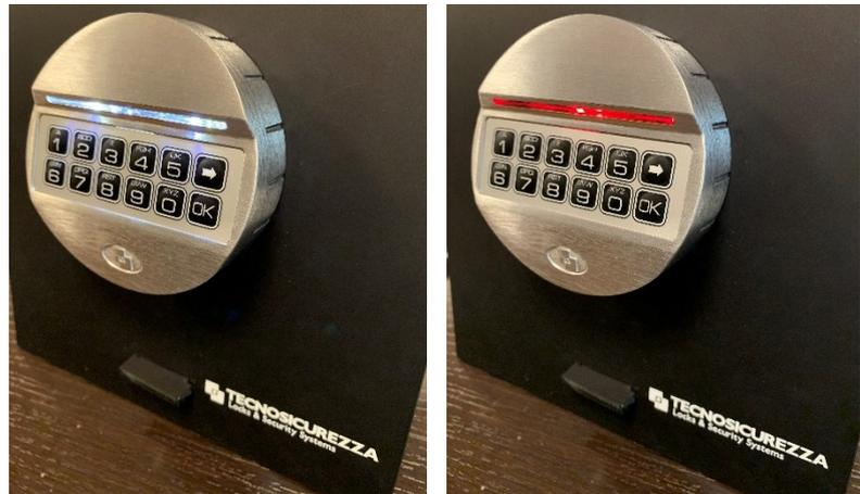
The thin transparent line incorporates in the central position also the red signalling LED normally present in all Pulse keypads.
